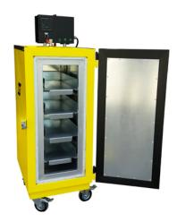
The SDE range of drying and storing ovens are large, thermally controlled cabinets designed specifically for welding electrodes. Ideally, a facility should have separate ovens for drying and storing. However with the SDE manual digital thermostat the same oven can be used for both drying and storing. Designed for stationary applications these come with heavy lockable castors to move around then lock in place. Aditionally a gas vent safely removes humidity and gases during the heating process.
